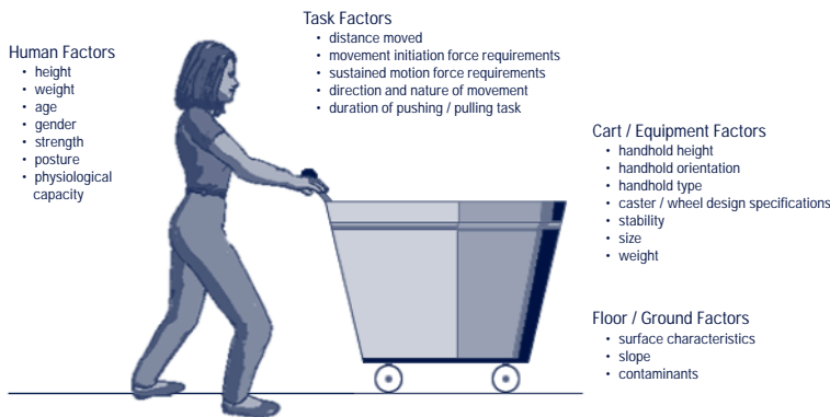
Figure 4. Some key factors that must be considered when designing a safe and productive pushing/pulling task, including human factors, task factors, cart and caster design, and floor and environmental conditions.
