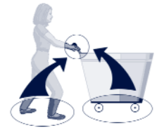
Figure 3. When people push wheeled equipment, they generate force and transmit that force through a contact point with the equipment. Friction at their feet must be at least equal to the resisting forces of the equipment, otherwise their feet will slip.
